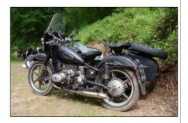
Above is Kamil Baran's Ural, with Keihin carbs, clever alternator drive, a Yamaha front wheel with disc brake, extra sump capacity with cartridge oil filter and a very exotic CMA cast rear wheel.
