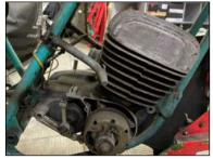
speed gearbox, gear primary drive and a much lighter flywheel. Usually these have two carbs but this one has only one, missing.
