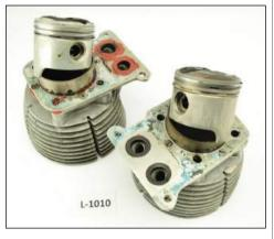
conversion plates screwed onto the bases to fit OHV barrels on a side valve.
