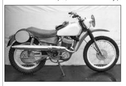
The text associated with this IZH 65M says "The next stage in the development of motorcycles for the USSR team was the IZH 65M developed in 1964. The engine tested on the IZH 60MS, boosted to 26 hp, combined with a new frame made of alloy steel 30HGSA. For the first time, plastics were widely used, from it fenders, saddle pan, headlight shroud and other parts were made. As a result, we
