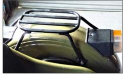
the original mudguard brackets on the inside and I drilled 2 holes in the light mounting for the outside fitting. Shown also is spare petrol tank and mounting to the rear of the sidecar which I made earlier. As the last couple of HV issues has had articles by Stephen Wood I thought it may be a good idea to show a photo of his and my Ural outfits. Stephens outfit originally belonged to David Angel and David used it for his own personal use.
